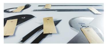
Randomly testing the sharpness of cutting edges emerging from centralized sharpening operations is a critical quality analysis that can significantly boost and maintain performance of cutting edges throughout your plant.
