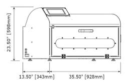
The work area diagram below shows the minimum space required for installation of the Sharpness Tester and its accessories, and takes into consideration operator safety, safe operation of the machine and test pieces, and access to machine for maintenance and cleaning.
